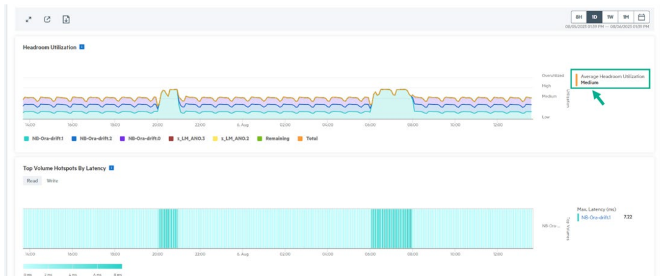
Figure 7. Headroom utilization and top volume hotspots in the HPE GreenLake for Block Storage performance dashboard
